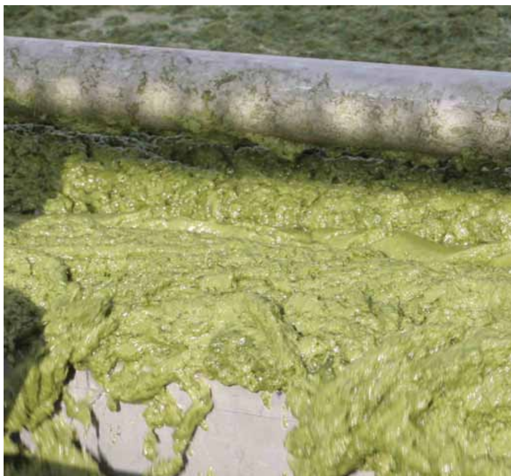
Figure 16: Algae and phosphorous after undergoing dissolved froth flotation. Phosphorus from the effluent of wastewater treatment ponds can be removed by chemical precipitation of the soluble phosphorous and then the solids, formed together with the algae, are separated from the water by flotation.
